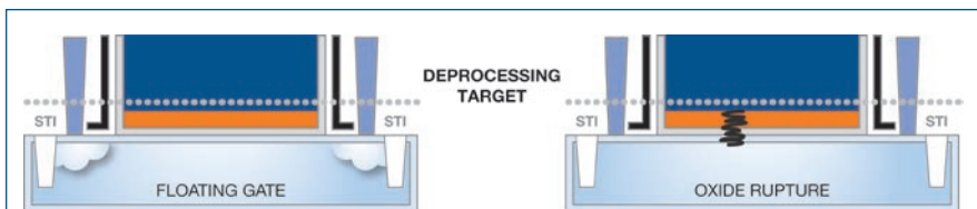
Figure 2 | Deprocessing is required for effective voltage contrast measurements.
