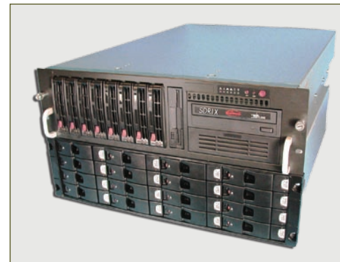
Figure 1 | Curtiss-Wright's SDR1X recorder is a rack-mounted system giving more than two hours of 10 GbE recording with options for SFPDP and 1 GbE links to the sensor.
